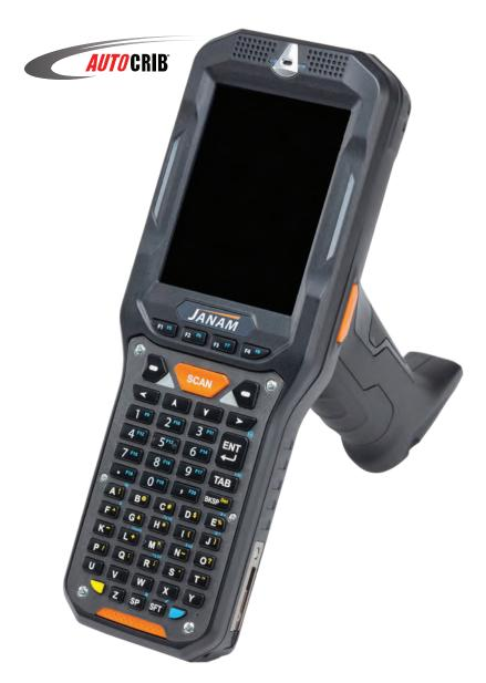
Our latest generation handheld, the MobileCrib, is built on the popular and simple to use Windows Mobile platform. It incorporates a high output laser scanner on the top of this feature rich unit.
